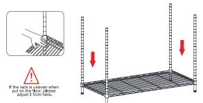
4 Install middle Tubes / top tubes accordingly.
